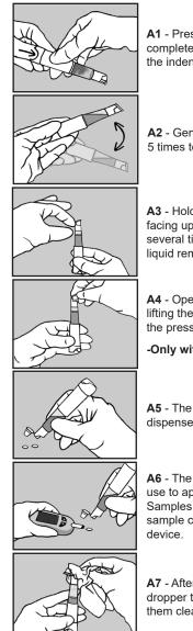
**A1** - Press the button firmly until it is completely pushed in and level with the indentation.
